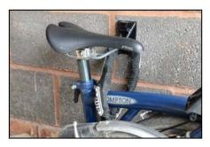
Wall bars and anchors can provide security for folding bicycles and may also be suitable for electric bikes.
