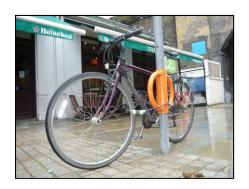
Wall bars (above left) should be secured with tamper-proof bolts. Hoops (above right) may be attached to suitable street furniture (with the approval of your local council).
